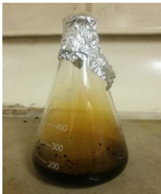
Figure S5: Pictorial image of waste tyre rubber crumb pre-treatment showing the yellowish-brown gas emitted during the process
