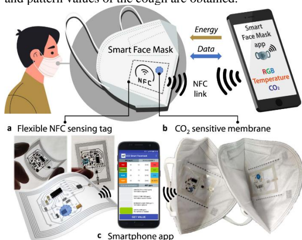
Fig. 3. A sample Architecture of a SFM with CO 2 monitoring capability (a) its NFC sensing tag (b) its CO 2 sensing layer (c) its smartphone application for support [30]
