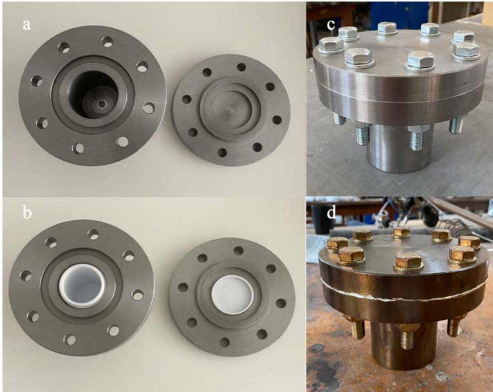
Figure A 4. Visualization of a) alloy steel vessel; b) vessel with the PTFE lining; c) top view of the assembled reactor; d) view of the reactor after running the first HTC test.
