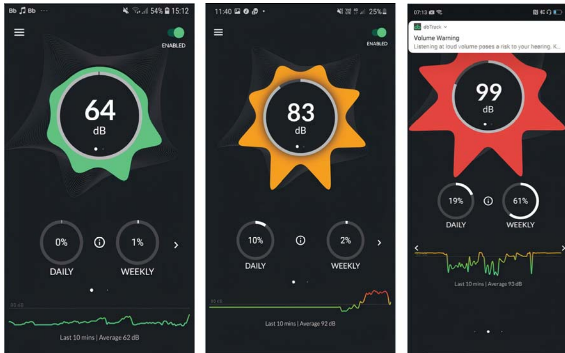
Figure 2. Green dbTrack application screen indicating safe listening (A), orange dbTrack application screen indicating moderate risk (B) and red dbTrack application screen indicating high risk with a volume warning (C).
