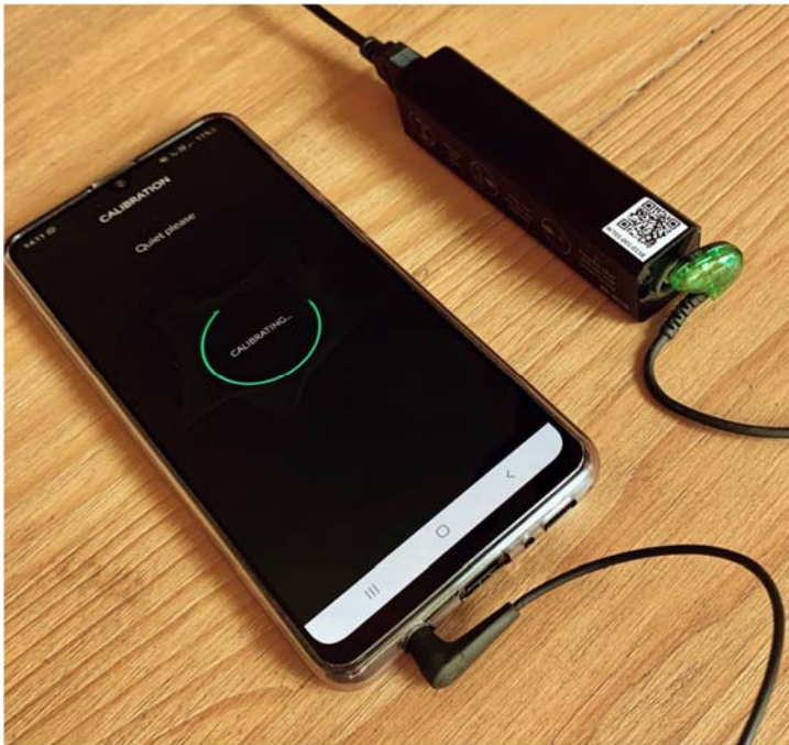
Figure 1. Calibration setup for the calibration of the in-ear microphone of the dbTrack sound-level monitoring earphones
