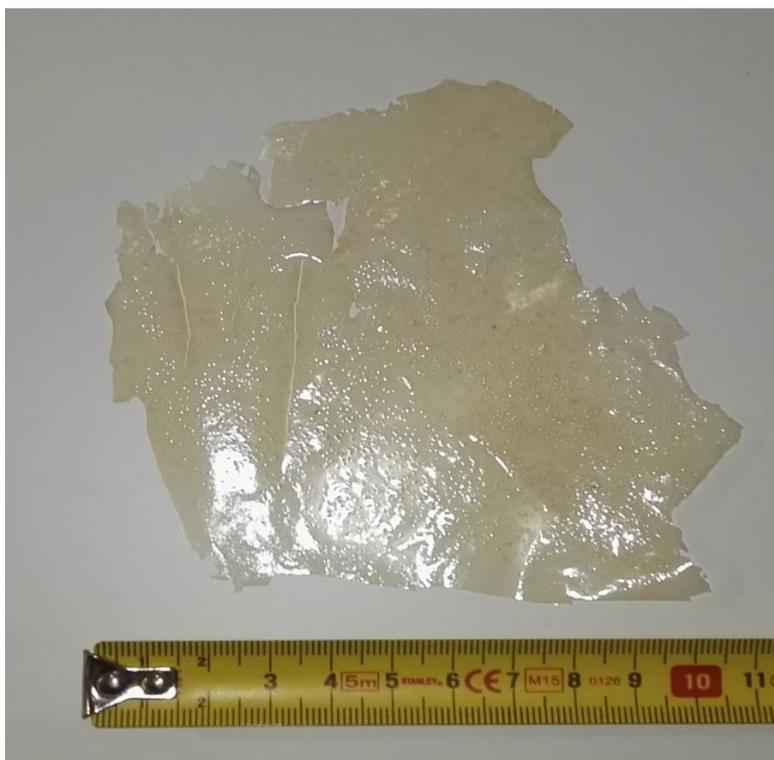
Figure 111: A broken qualitative film produced without dewatering KEMS
