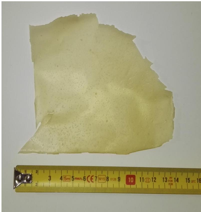
Figure 114: A broken qualitative film produced from agglomerated microparticles
