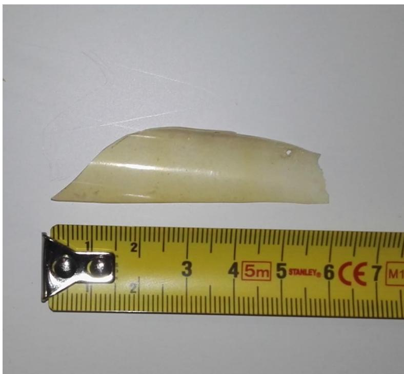
Figure 112: A broken shard of thick film produced without dewatering KEMS
