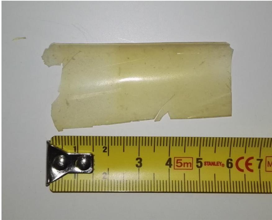
Figure 113: Another broken piece of thick film produced from KEMS
