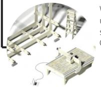
Wikihouse allows for the manufacturing of an entire house's structure with no more than a CNC machine.
