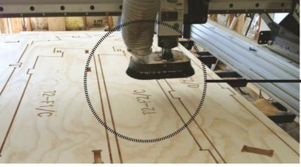
All components are labelled through the CNC process and allows for construction to take place similarly to a Lego set.
