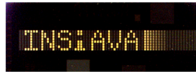
Fig. 12 An optical micrograph of the dot matrix display clearly shows the active pixels when illuminated.
