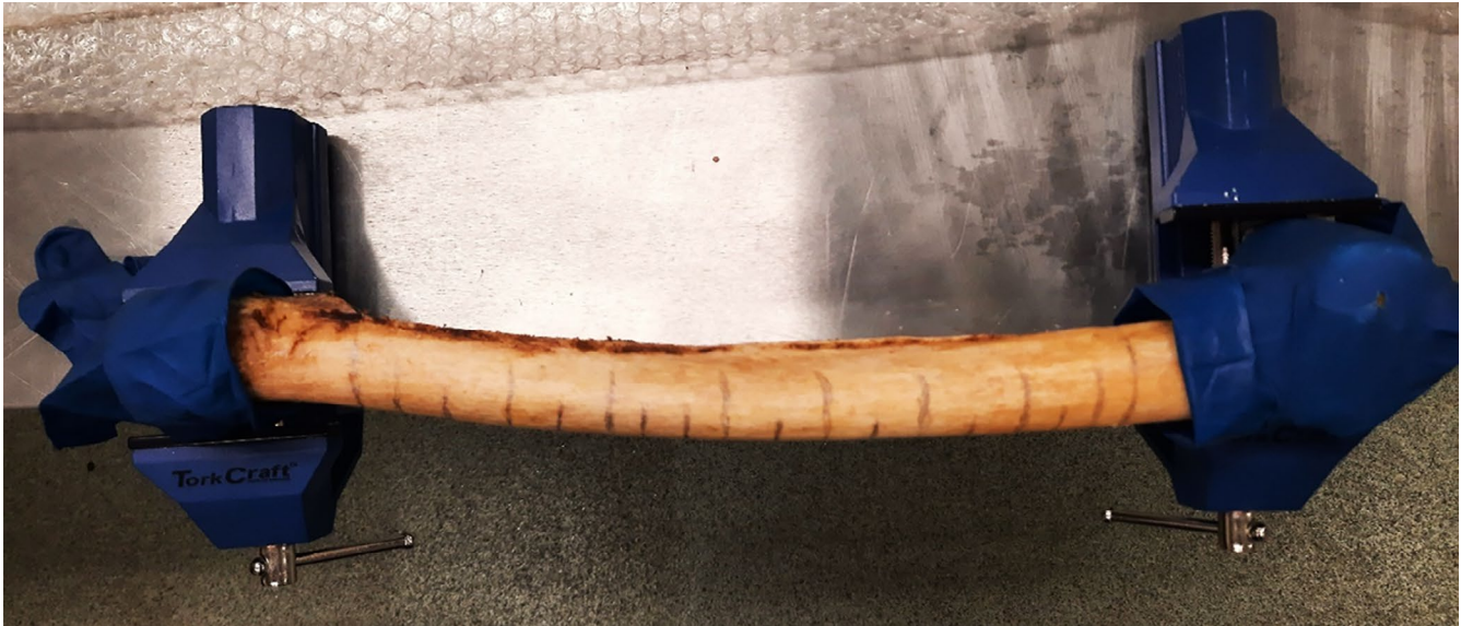
FIGURE 1 Double bench vice setup to clamp the femur at the proximal (left) and distal (right) ends.
