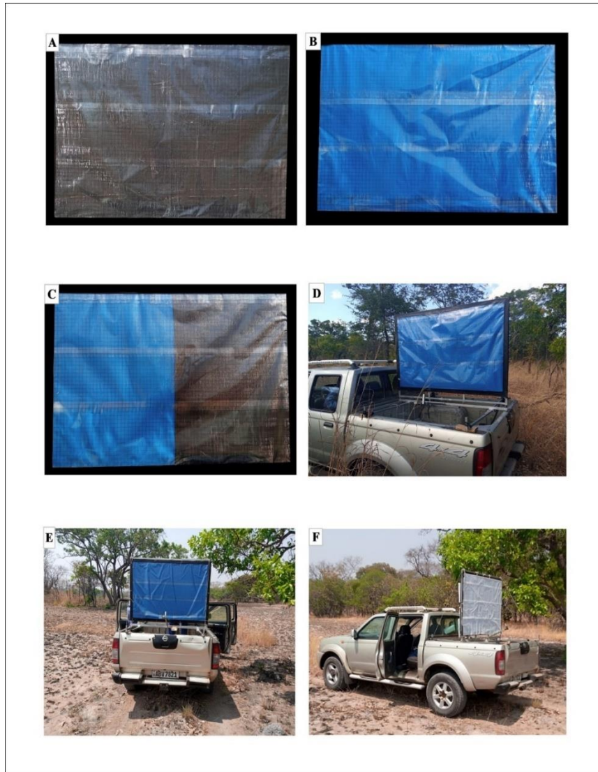
Fig 2.1: Vehicle-mounted sticky panel traps. (A) All-black sticky panel trap. (B) All-blue sticky panel trap. (C) 1:1 blue-black sticky panel trap. (D) All-blue sticky panel trap mounted in-line orientation (E) All-blue sticky panel trap mounted in transverse orientation (F) All-blue sticky panel in transverse orientation covered with non-stick baking paper.
