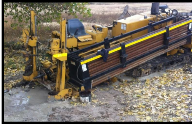
Figure 6: Horizontal Directional Earth Drilling Machine (Author's Own Source).
