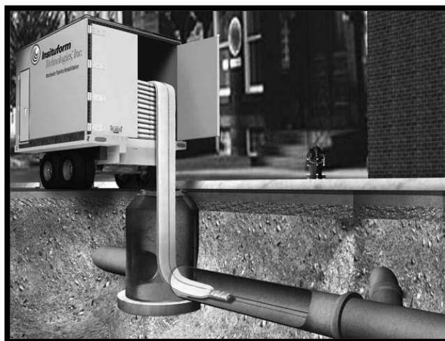
Figure 26: Cured-In-Place Process (Najafi, 2010: 58)
