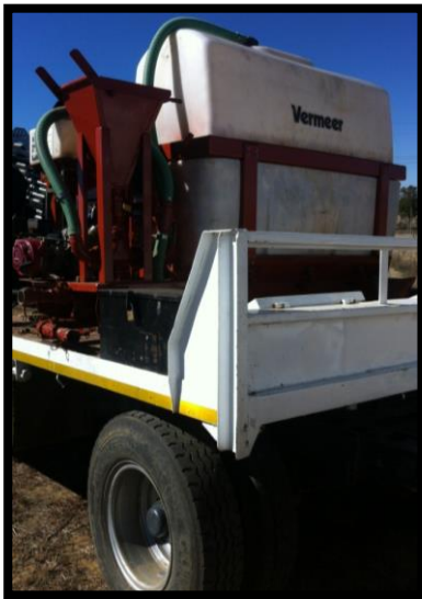
Figure 8: Drilling Fluid Mixing System for HDD (Author's Own Source).
