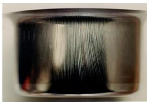
Figure 2-6: Ridging on an AISI FSS sink [41].
