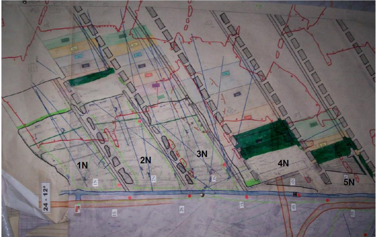
Fig. S1. UG2 panels mined toward and below a Merensky remnant.
