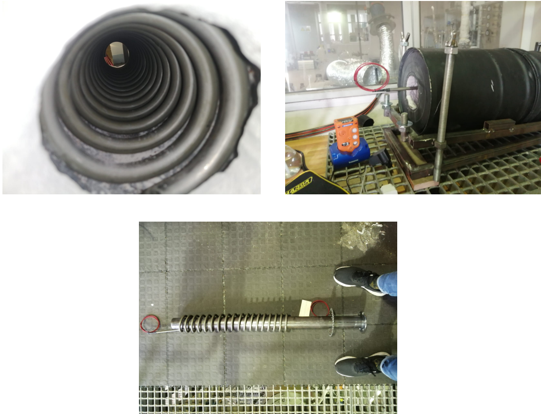
Figure 3.9: 5.5 kW Heating element, inside the insulation (top left), external to the reactor (top right) and curled around the kiln tube (bottom).
