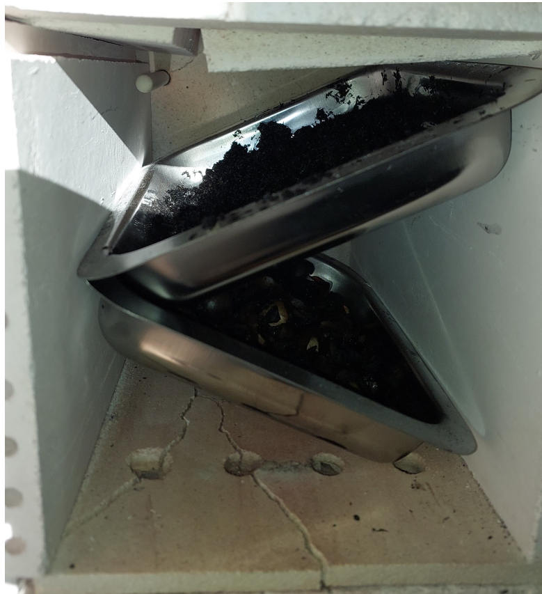
Figure 3.22: Produced biochar samples drying in kiln at 105 °C.
