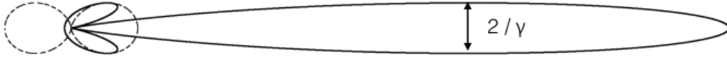
FIGURE 2.8: In the frame of the electron, the dipole radiation power pattern is shown by the dotted line. However, in the frame of the observer, the transformed pattern is shown by the solid line with a width \theta = 2/\gamma for \gamma \gg 1 . Taken from Condon and Ransom (2016).
