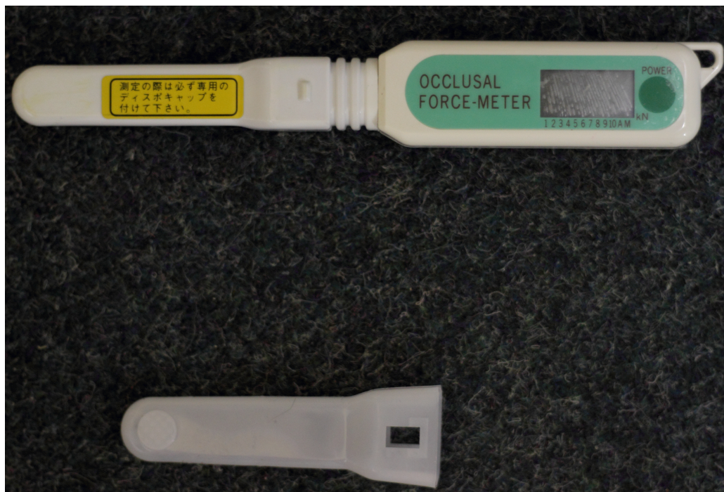
Figure 14: Close up of meter, with sterile casing
