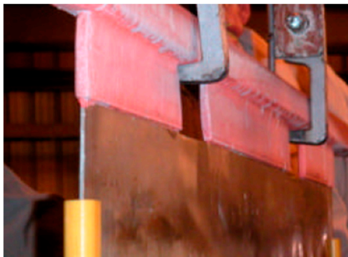
Figure 5. ISA cathode BR in service at Compañía Minera Zaldívar, Chile (Figure 1 from [12] in the Proceedings of Copper 2003 5th International Conference, Vol. 5. Reprinted with permission of the Canadian Institute of Mining, Metallurgy and Petroleum).
