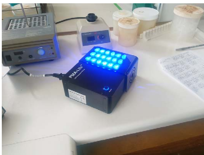
Figure 4.1: Photoactivation on a PMA-Lite™ LED Photolysis Device.
