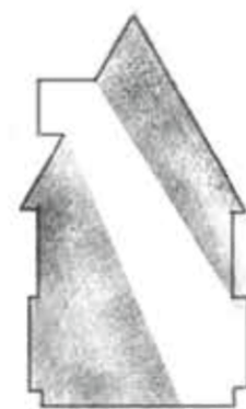
Roof articulations provide light to the indoor environment
