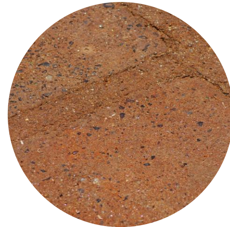
Figure 21: Ferrock surface and texture (Author, 2024)
