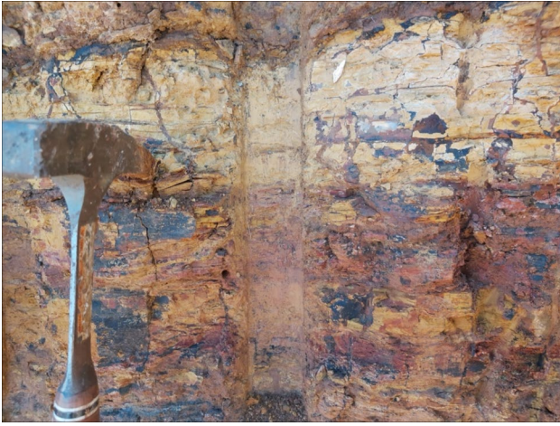
Fig. 17 Photograph taken of completely weathered andesite sample 2835 (photographs taken by D Swart)
