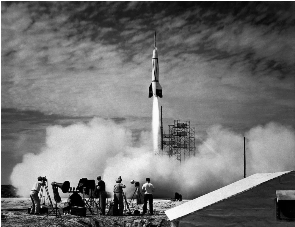
Figure 29: The German V2 rocket was the world's first large-scale liquid-propellant rocket developed between 1936 and 1942 in Nazi Germany. Credit: Getty Images (Harvey 2022).
