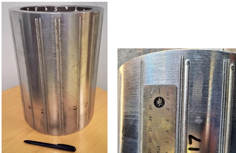
Fig. 4.4 Images of preliminary laser beads of different elements deposited on the seamless P91 steel pipe.
