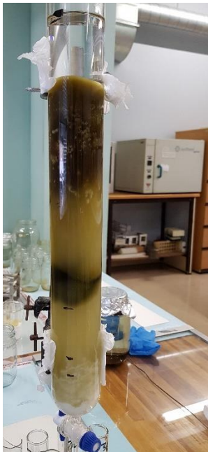
Figure 5.2 Silica gel chromatography of the pooled non-polar fractions obtained from SSF of the P. zombamontana acetone leaf extract.
