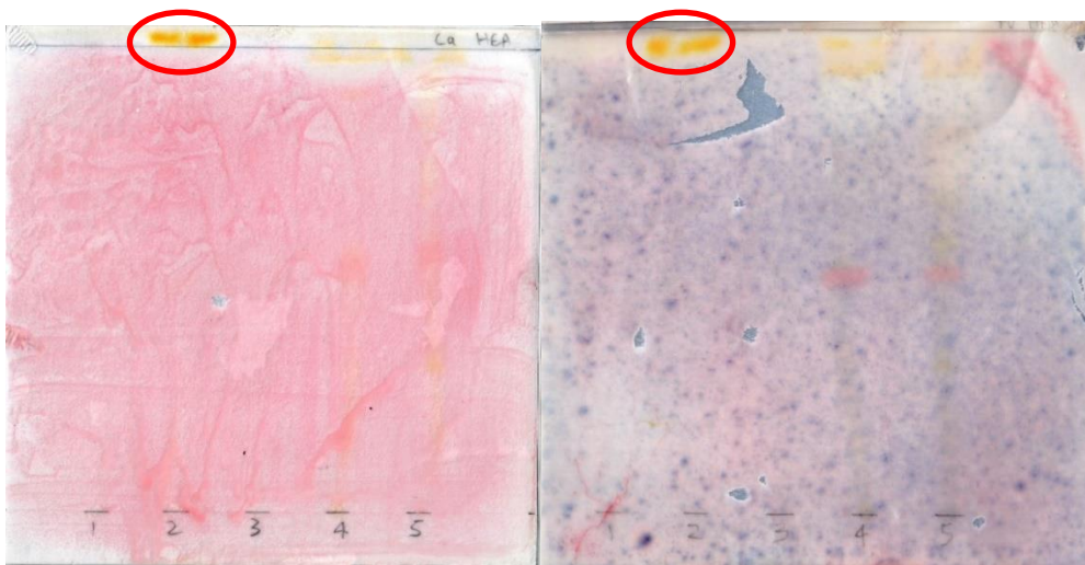
Figure 5.5 Bioautogram of sub-fractions 1-5, with C. albicans (left) and F. verticillioides (right). The clear zones marked represent inhibition zones and therefore the presence of an active compound.
