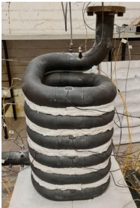
Fig. 6. Receiver with ceramic fibre blanket between coils.
