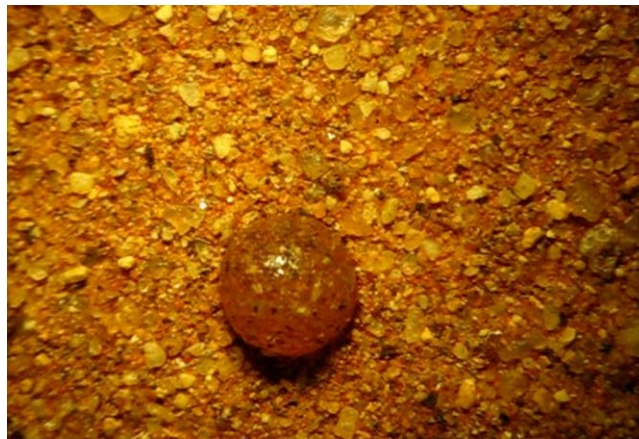
Figure 3.6 A water drop placed on soil collected from within FC displaying a decrease in the ease of wettability of the soil sample
