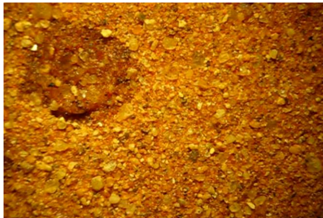
Figure 3.5 The WDPT test performed on matrix soil. The dampened location in the image above displays the position where the water drop was placed
