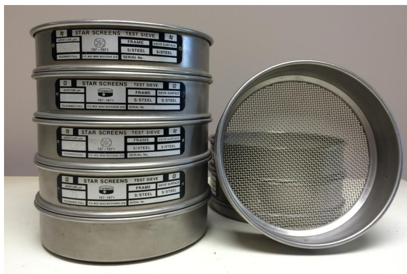
Figure 3.1 Stacked sieves with various aperture sizes used for soil texture analysis
