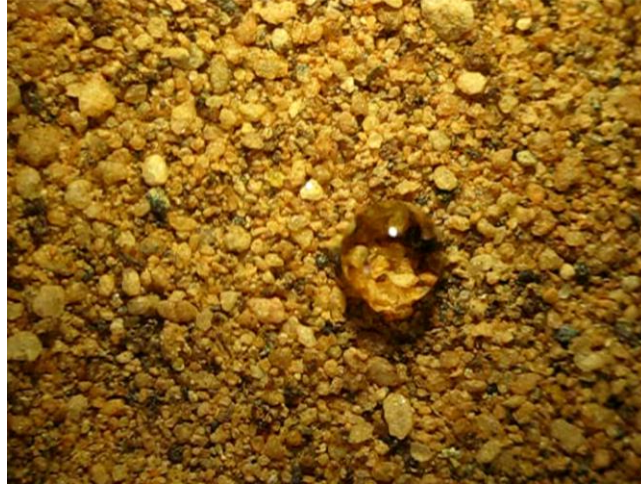
Figure 3.7 A water drop placed on soil collected from decomposing plant location indicating extreme resistance to penetration
