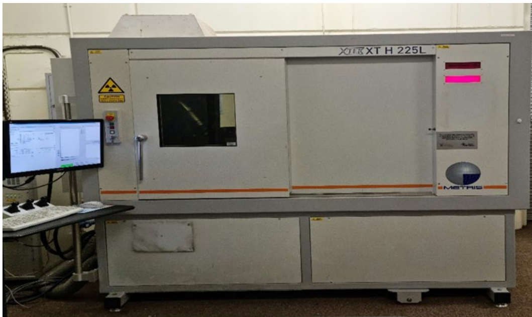
Figure 3. XTH 225 ST micro-focus X-ray tomography system (Nikon) at the MIXRAD Facility
