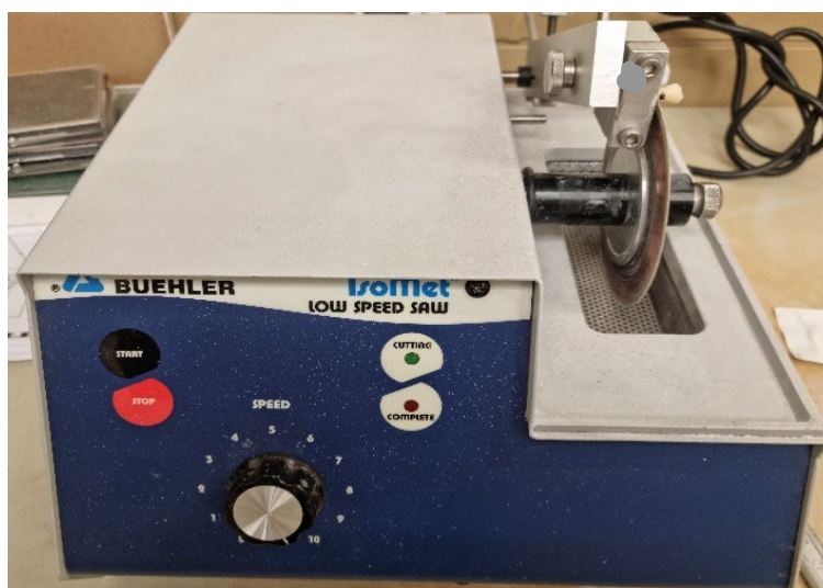
Figure 5. ISOMET™ low-speed precision cutter
