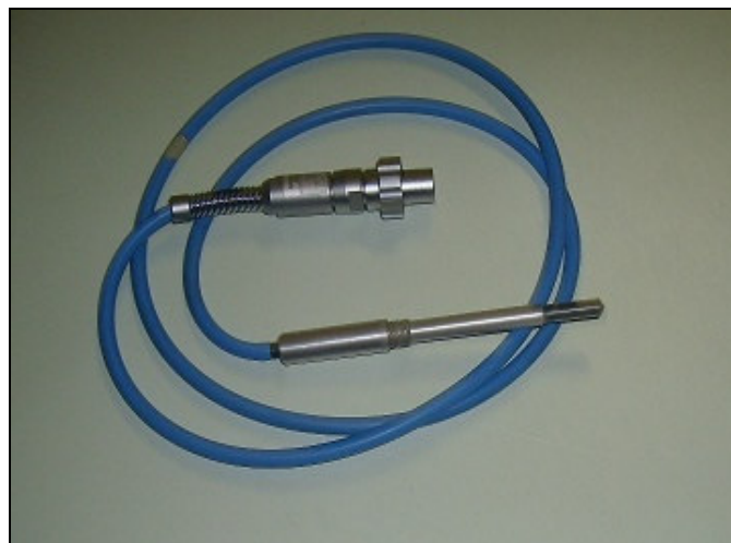
Figure 6.3. The Farmer ionization chamber that was used for the absolute dose measurements.
