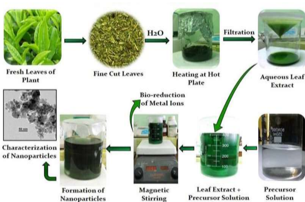
Figure 2.9: Mapping of environmentally friendly synthesis method using plant leaves for the production of NPs [67].
