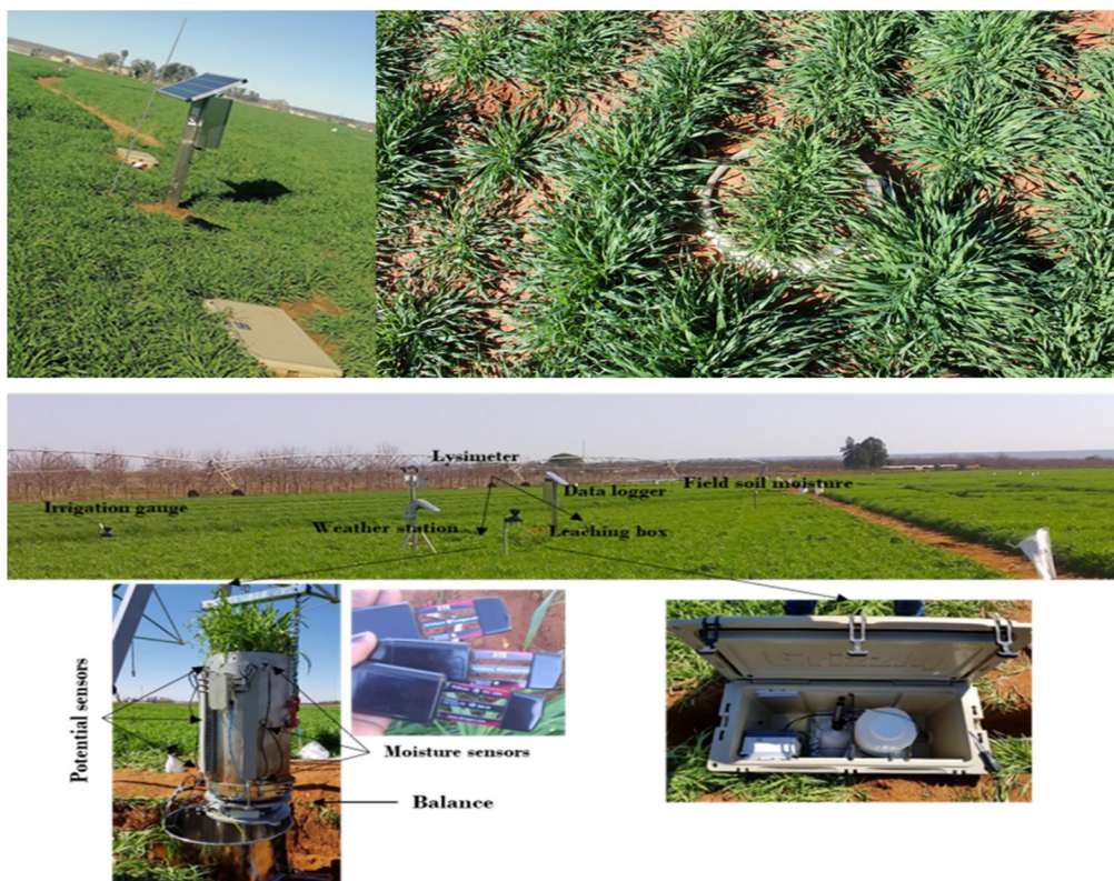
Figure 2. A view of the field experimental setting of the lysimeter and meteorological station.
