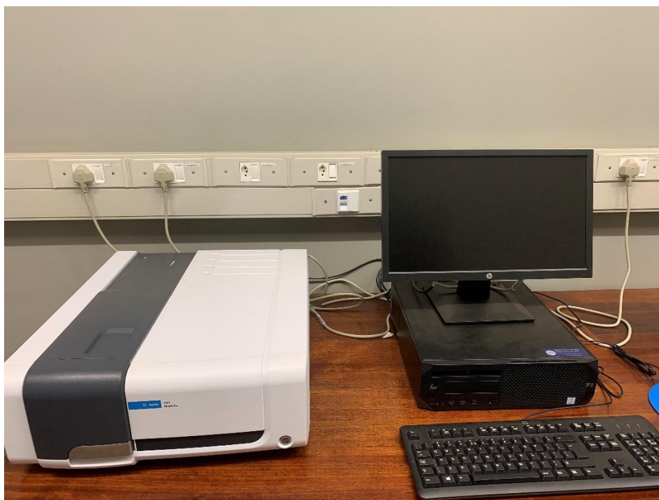
Figure 3.6.9. Photograph of the UV-Vis spectrometer used in this study.
