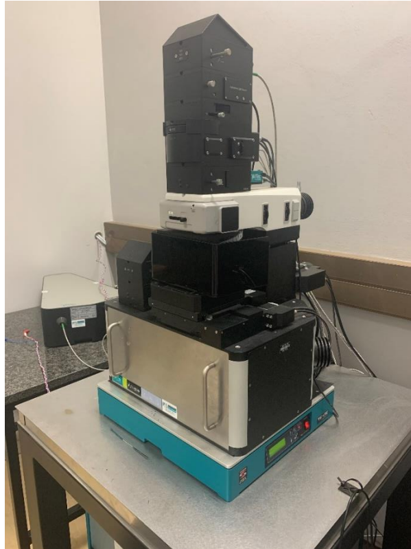
Figure 3.6.5. Photograph of the WITec alpha300 RAS+ Raman spectroscopy setup used in this study.
