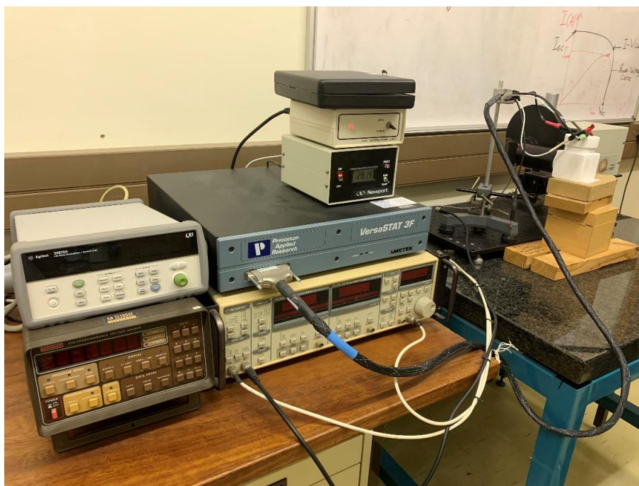
Figure 3.6.11. Photograph of the electrochemical setup including the VersaSTAT 3F potentiostat as used in this study.
