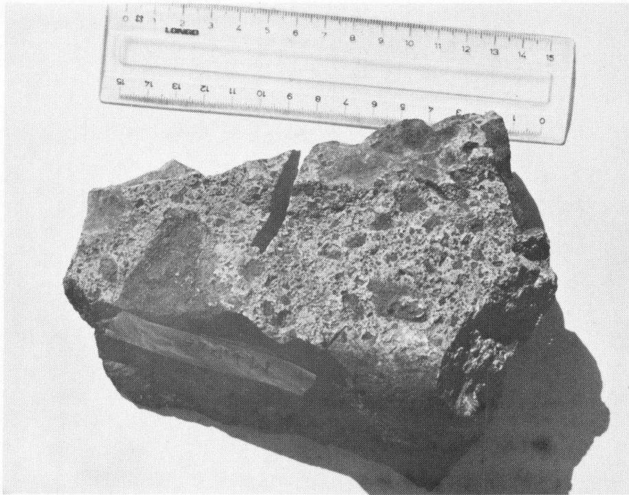
Fig. 4 – Volcanic breccia with dark angular fragments of various sizes in a light, cream-coloured, fine-grained felsitic groundmass
