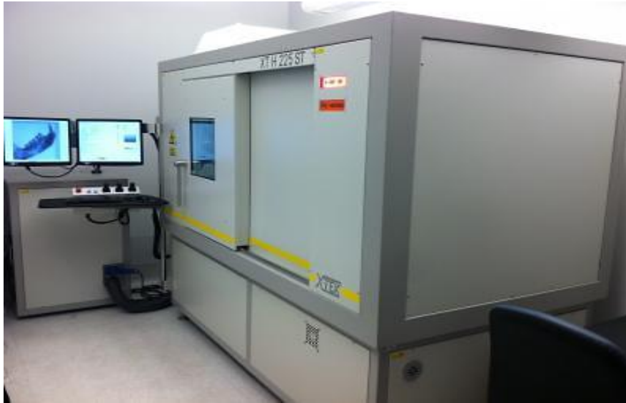
Figure 3.16: XTH 225 ST micro-focus X-ray tomography system (Nikon) at the MIXRAD facility (Photo courtesy of Hoffman et al. 112 )
