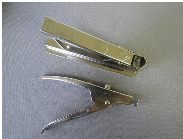
Figure 3.4: Capsule activator used with 3M ESPE products (top) and applicator used with all products tested (below)
