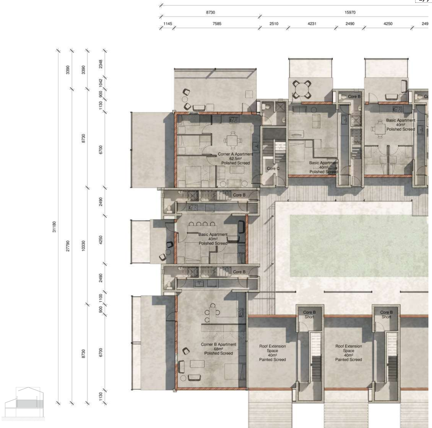
Figure 177 The final iteration of the first floor plan.
