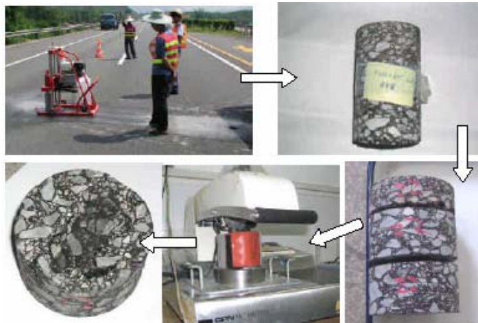
Figure 7. Wheel tracking test procedure of cut core samples.
