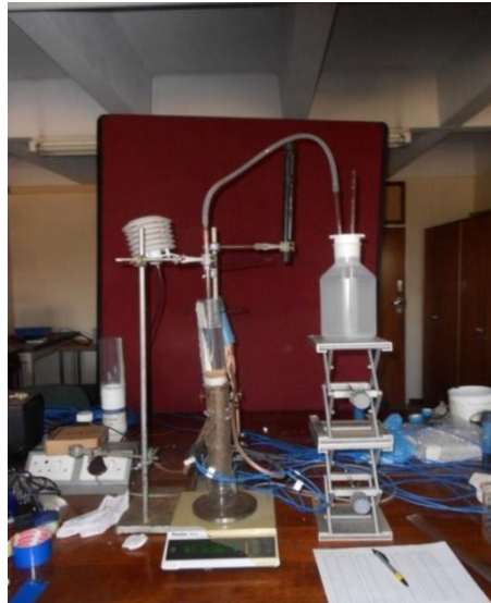
Figure 0.1 Initial experimental set-up for the calibration of sap flow techniques using the stem perfusion method
