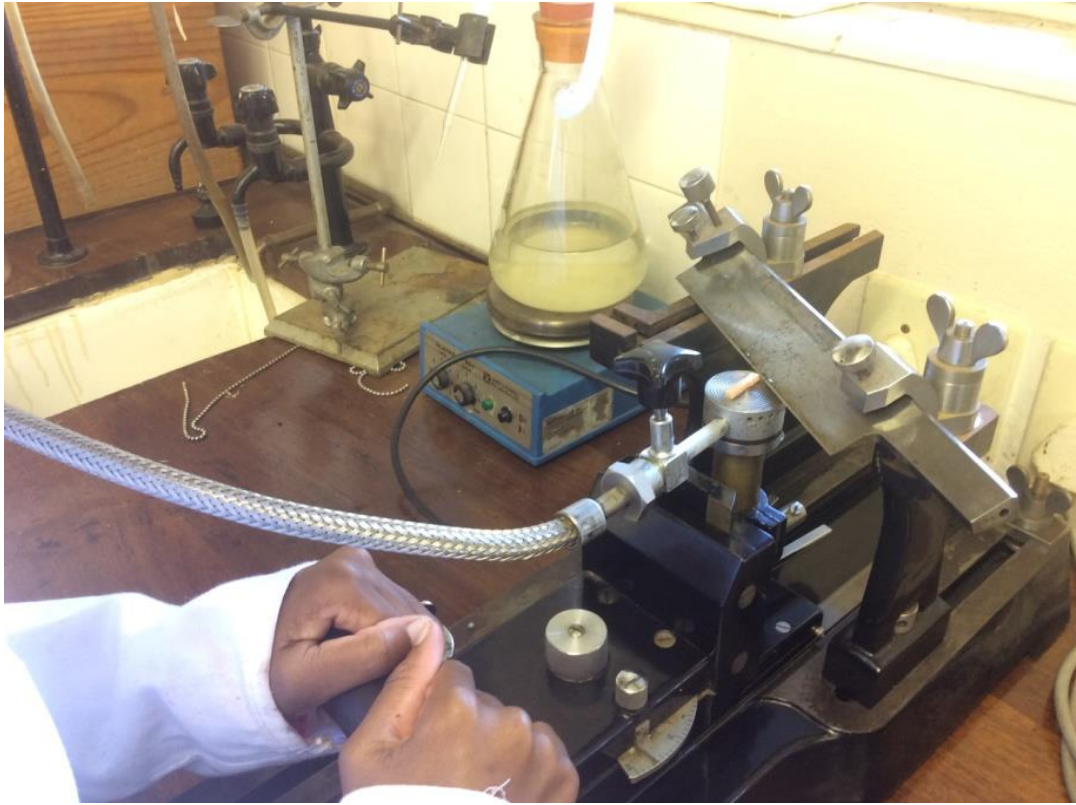
Figure 0.6 Cutting of sections using the sliding microtome
