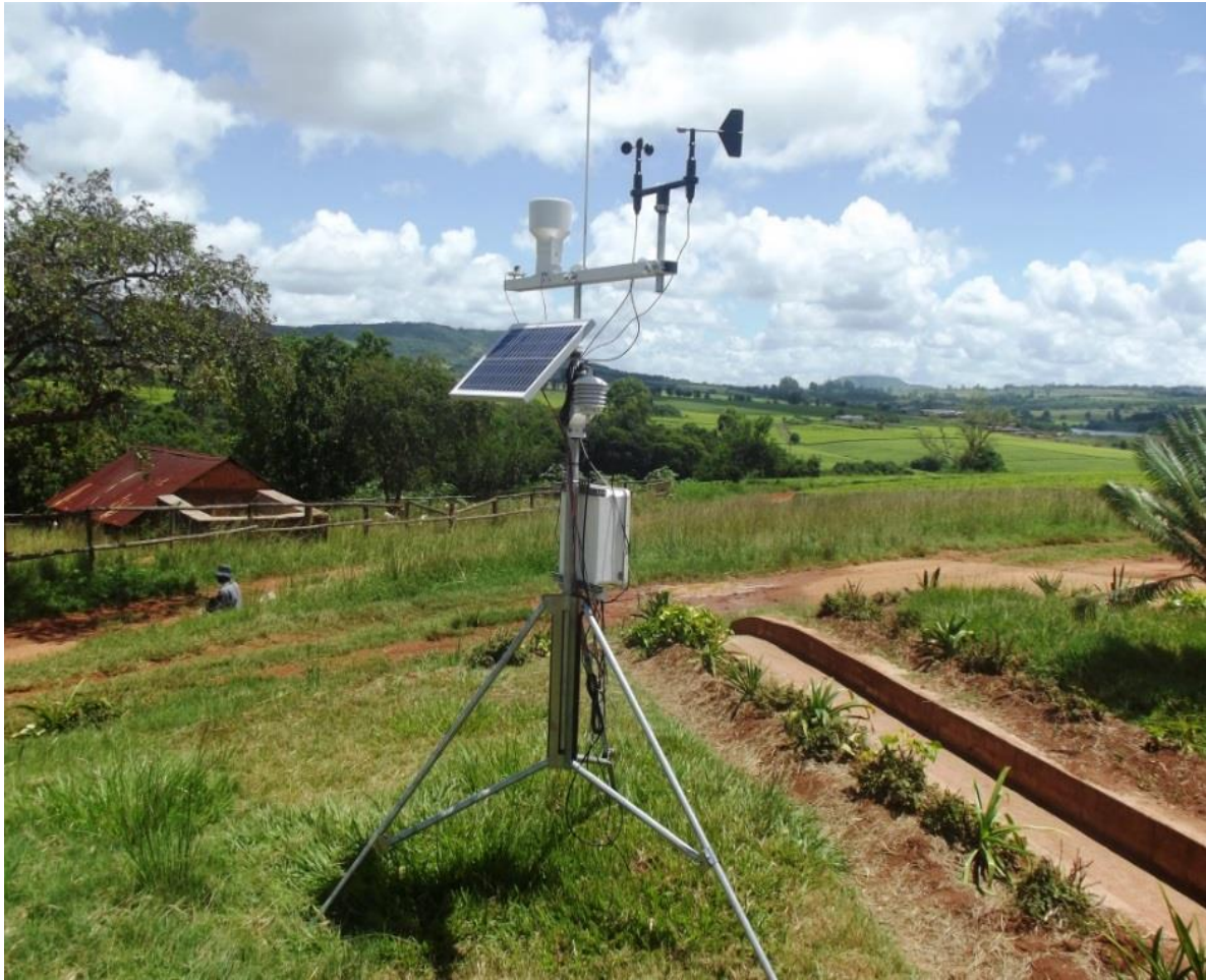
Figure 3.5 Campbell Scientific Automatic weather station installed at the study site for the period 2010-2013
