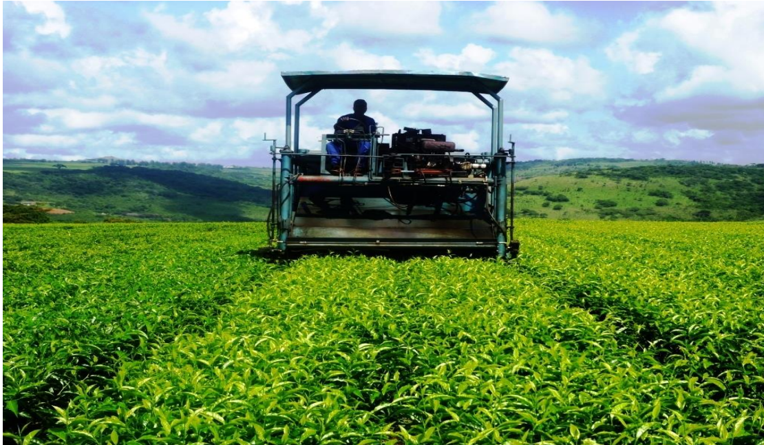
Figure 2. 7 Ride–on self-propelled tea harvester at Tingamira estate (Photo: by Madamombe, June 2011)
