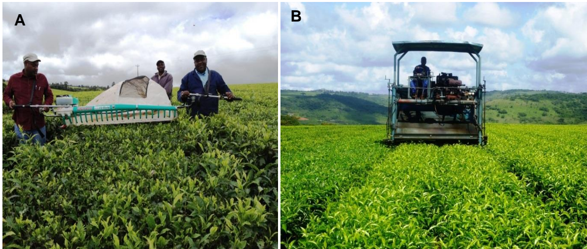
Figure 3.2 Mechanical harvesting machines, which included (A) the hand-held Ochiai, and (B) the ride-on self-propelled tea harvester.
