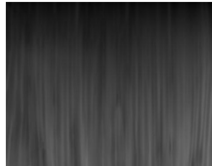
Figure 3: Instantaneous temperature distribution of the foil underside illustrative of the flow thermal traces as obtained by the FLIR SC3000 camera at conditions of Re = 360 , heat flux of 2.1 \text{ Wcm}^{-2} and pulsation frequency of 1.76 Hz. The vertical axis corresponds to the stream-wise direction while the horizontal to the span-wise direction. From dark to bright, the colour scale represents cool to hotter regions.
