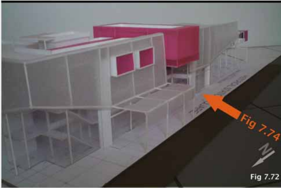
Fig 7.72 again shows a view from the North-Western Corner of the building, towards the South-East. The building is now wrapped in a 'skin' that serves not only to protect it from the harsh sun, but also to unify the different functions expressed in the facade. This shading 'skin' is perforated, allowing diffused light to penetrate the building. Combined with the hovering auditorium, it adds to the building's quality of lightness. The North-Western Corner is subtly defined by the meeting of this shading 'skin's diagonal lines. The protrusion of the conference through the 'skin' breaks the surface and creates a focal point of the Western facade. (photo by author)
