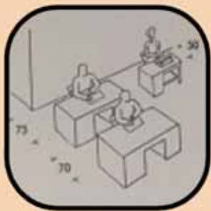
Fig 7.126 Circulation space required in offices. (Neufert 1970)
