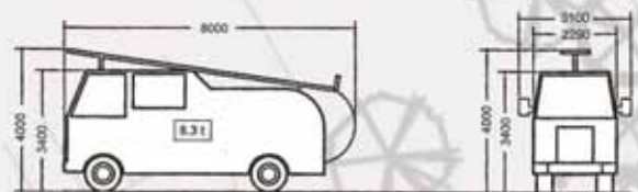
Fig. 8.123 above show a medium sized fire fighting vehicle's dimensions (Adler 2001:4-2)
