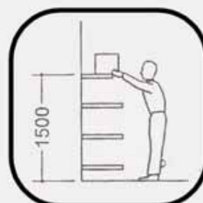
Fig 7.138 shows the position of a shelf on eye level. (Adler 1999:18-9)
