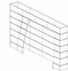
Internal plexiglas infill panels
